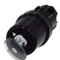
Key-operated switch BKS, 22 mm, round, plastic, Lock No. E9 (VW), without key, 2 switch positions O-I, latching, actuating angle  $90^{\circ}$ , 10:30h/13:30h, Key removal O
