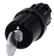
Key-operated switch BKS, 22 mm, round, plastic, Lock No. E2 (VW), without key, 3 switch positions I-O-II, latching, actuating angle 2x45°, 10:30h/12h/13:30h, Key removal I+O+II
