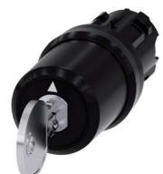
Key-operated switch BKS, 22 mm, round, plastic, lock number S1, with 2 keys, 3 switch positions I>O<II, momentary contact on the left, latching on the right, actuating angle  $2x45^{\circ}$ , 10:30h/12h/13:30h, Key removal O
