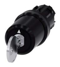
Key-operated switch BKS, 22 mm, round, plastic, lock number S1, with 2 keys, 3 switch positions I-O<II, left latching, right momentary contact type, actuating angle 2x45°, 10:30h/12h/13:30h, Key removal I
