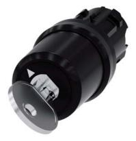
key-operated switch Siemens, 22 mm, round, plastic, lock no. LSG1, with 2 keys, 2 switch positions O<I, momentary contact type, actuating angle  $45^\circ,\,10:30h/12h,$  key removal O
