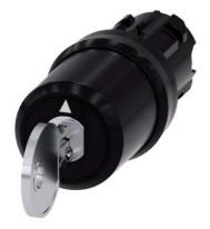
key-operated switch Siemens, 22 mm, round, plastic, lock number SSG10, with 2 keys, 3 switch positions I-O<II, left latching, momentary contact type on the right, actuating angle  $2x45^\circ$ , 10:30h/12h/13:30h, key removal I
