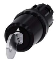
key-operated switch Siemens, 22 mm, round, plastic, lock number SSG10, with 2 keys, 3 switch positions I-O-II, latching, actuating angle 2x45°, 10:30h/12h/13:30h, key removal II
