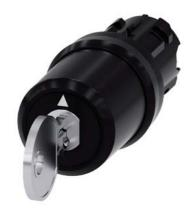
key-operated switch Siemens, 22 mm, round, plastic, lock number SSG10, with 2 keys, 3 switch positions I-O-II, latching, actuating angle 2x45°, 10:30h/12h/13:30h, key removal I+O+II
