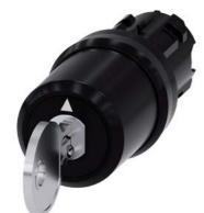
key-operated switch Siemens, 22 mm, round, plastic, lock number SSG10, with 2 keys, 3 switch positions I-O-II, latching, actuating angle  $2x45^{\circ}$ , 10:30h/12h/13:30h, key removal O
