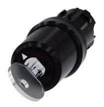
key-operated switch Siemens, 22 mm, round, plastic, lock number SSG10, with 2 keys, 2 switch positions O-I, latching, actuating angle 90°, 10:30h/13:30h, key removal O
