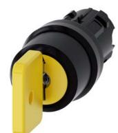
Key-operated switch O.M.R, 22 mm, round, plastic, lock number 73033, yellow, with 2 keys, 3 switch positions I-O-II, latching, actuating angle 2x45°, 10:30h/12h/13:30h, Key removal I+O+II
