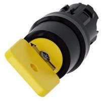
Key-operated switch O.M.R, 22 mm, round, plastic, lock number 73033, yellow, with 2 keys, 2 switch positions O-I, latching, actuating angle  $90^\circ$ , 10:30h/13:30h, Key removal O+I
