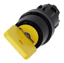
Key-operated switch O.M.R, 22 mm, round, plastic, lock number 73033, yellow, with 2 keys, 2 switch positions O<I, momentary contact type, Actuating angle 45°, 10:30h/12h, Key removal O
