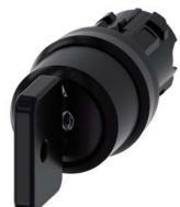
Key-operated switch O.M.R, 22 mm, round, plastic, lock number 73034, black, with 2 keys, 3 switch positions I-O<II, left latching, right momentary contact type, actuating angle 2x45°, 10:30h/12h/13:30h, Key removal I
