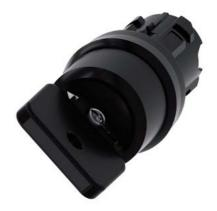
Key-operated switch O.M.R, 22 mm, round, plastic, lock number 73034, black, with 2 keys, 2 switch positions O-I, latching, actuating angle 90°, 10:30h/13:30h, Key removal I
