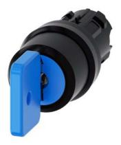
Key-operated switch O.M.R, 22 mm, round, plastic, lock number 73038, blue, with 2 keys, 3 switch positions I-O<II, left latching, right momentary contact type, actuating angle  $2x45^{\circ}$ , 10:30h/12h/13:30h, Key removal O
