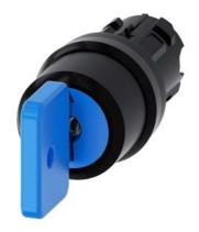
Key-operated switch O.M.R, 22 mm, round, plastic, lock number 73038, blue, with 2 keys, 3 switch positions I-O-II, latching, actuating angle  $2x45^\circ,\,10:30h/12h/13:30h,$  Key removal I+O+II
