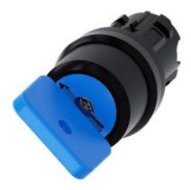
Key-operated switch O.M.R, 22 mm, round, plastic, lock number 73038, blue, with 2 keys, 2 switch positions O-I, latching, actuating angle  $90^\circ$ , 10:30h/13:30h, Key removal O+I
