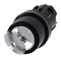
RONIS key-operated switch, 22 mm, round, plastic, Lock No. 421, with 2 keys, 2 switch positions O-I, latching, actuating angle  $90^\circ$ , 10:30h/13:30h, Key removal O+I
