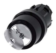
RONIS key-operated switch, 22 mm, round, plastic, lock number 455, with 2 keys, 2 switch positions O<I, momentary contact type, Actuating angle 45°, 10:30h/12h, Key removal O
