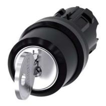
RONIS key-operated switch, 22 mm, round, plastic, lock number SB30, with 2 keys, 3 switch positions I>O-II, momentary contact on the left, latching on the right, actuating angle 2x45°, 10:30h/12h/13:30h, Key removal II, possible special locks: SB31, 421, 455
