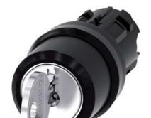
RONIS key-operated switch, 22 mm, round, plastic, lock number SB30, with 2 keys, 3 switch positions I-O<II, left latching, right momentary contact type, actuating angle 2x45°, 10:30h/12h/13:30h, key removal I, possible special locks: SB31, 421, 455
