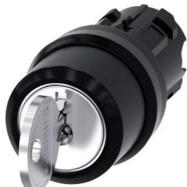
RONIS key-operated switch, 22 mm, round, plastic, lock number SB30, with 2 keys, 3 switch positions I-O-II, latching, actuating angle 2x45°, 10:30h/12h/13:30h, Key removal I+O+II, possible special locks: SB31, 421, 455
