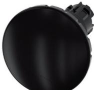
Mushroom pushbutton, 22 mm, round, plastic, black, 60 mm, positive latching, acc. to EN ISO 13850, rotate-to-unlatch
