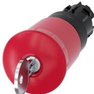
EMERGENCY STOP mushroom pushbutton, 22 mm, round, plastic, red, 40 mm, with lock Siemens, lock no. SSP9, positive latching, according to DIN EN ISO 13850, key-operated release
