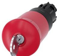
EMERGENCY STOP mushroom pushbutton, 22 mm, round, plastic, red, 40 mm, with lock BKS, lock No. E9 (VW), positive latching, acc. to EN ISO 13850, keyoperated release, supplied without key
