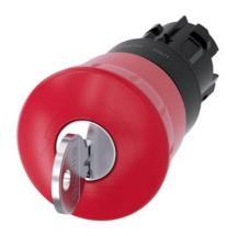
EMERGENCY STOP mushroom pushbutton, 22 mm, round, plastic, red, 40 mm, with RONIS lock, lock number SB30, positive latching, acc. to EN ISO 13850, key-operated release
