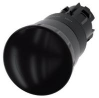
Mushroom pushbutton, 22 mm, round, plastic, black, 40 mm, positive latching, acc. to EN ISO 13850, rotate-to-unlatch
