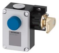
Cable-operated switch and lever Metal enclosure, 2 x M25 x 1.5; 1 NO+1 NC, latching EN ISO 13850 and pushbutton release, 2-sided operation, for wire lengths up to 2 x 100 m
