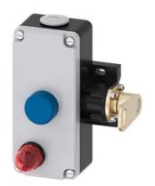
Cable-operated switch and lever Metal enclosure, 2 x M25 x 1.5; 2 NO+2 NC, latching according to EN13850 and pushbutton release with LED lamp red DC 24 V, 2-sided operation, for wire lengths up to 2 x 100 m
