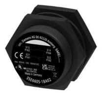
magnetically-operated switch contact block, round M30 contacts 1 NC/1 NO with M12 plug 4-pole Pin1=21, Pin2=22 Pin3=13, Pin4=14. Required solenoid 3SE6704-1BA. coupling with connection cable 5 m 3SX5601-3SB54
