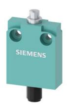
Position switch in compact design 40 mm wide with connector plug M12 Snapaction contacts 1 NO+1 NC with rounded plunger
