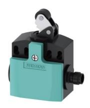
Position switch Plastic enclosure, 50 mm Device connection 2 x (M20 x 1.5) 1 NO/2 NC quick action contacts with M12 connector, 4-pole on the right, 2 NC connected Pin assignment: Pin1=21, Pin2=22 Pin3=31, Pin4=32 max. 250 V and 4 A Roller lever with plastic roller 13 mm
