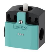
Position switch Plastic enclosure according to EN 50047, 50 mm Device connection 2 x (M20 x 1.5) 1 NO/2 NC quick action contacts LEDs 110-230 V AC, yellow/green Teflon plunger
