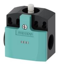
Position switch Plastic enclosure according to EN 50047, 50 mm Device connection 2 x (M20 x 1.5) 1 NO/2 NC slow-action contacts LEDs 110-230 V AC, yellow/green Teflon plunger
