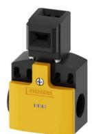
Safety position switch with separate actuator Plastic enclosure, 50 mm Device connection 2x (M20x 1.5) Slow-action contacts 1 NO+2 NC with 2 LEDs yellow/green 24 V DC 5 directions of approaches The matching separate actuator 3SE5000-0AV0. must be ordered separately
