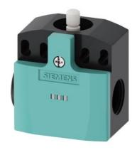
Position switch Plastic enclosure, 50 mm according to EN 50047 Device connection 2 x (M20 x 1.5) 1 NO/2 NC quick action contacts LED, yellow/green, 24 V DC Teflon plunger
