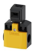
Safety position switch with separate actuator Plastic enclosure, 50 mm Device connection 2x (M20x 1.5) Slow-action contacts 1 NO+1 NC 5 directions of approaches Pull-out force 30 N The matching separate actuator 3SE5000-0AV0. must be ordered separately
