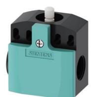
Position switch with increased corrosion protection Plastic enclosure wide, according to EN 50047, 50 mm Device connection 2 x (M20 x 1.5) 2 NO/1 NC slow-action contacts Teflon plunger
