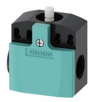
position switch plastic enclosure according to EN 50047, 50 mm device connection 2 x (M20 x 1.5) 1 NO/2 NC slow-action contacts with make-before-break rounded plunger
