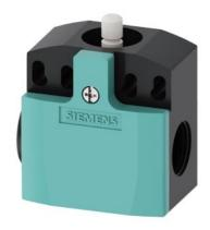
Position switch with increased corrosion protection Plastic enclosure wide, according to EN 50047, 50 mm Device connection 2 x (M20 x 1.5) 1 NO/2 NC slow-action contacts with make-before-break Teflon plunger
