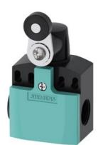
Position switch Plastic enclosure according to EN 50047, 50 mm Device connection 2 x (M20 x 1.5) 1 NO/2 NC quick action contacts twist lever right/left adjustable with plastic roller 19 mm
