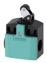
Position switch Plastic enclosure according to EN 50047, 50 mm Device connection 2 x (M20 x 1.5) 1 NO/2 NC quick action contacts Roller lever with plastic roller 13 mm
