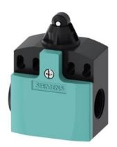
Position switch Plastic enclosure according to EN 50047, 50 mm Device connection 2 x (M20 x 1.5) 1 NO/2 NC quick action contacts Roller plunger with plastic roller 10 mm
