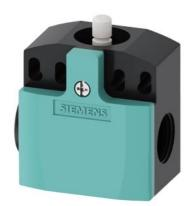
Position switch with increased corrosion protection Plastic enclosure wide, according to EN 50047, 50 mm 1 NO/2 NC quick action contacts Teflon plunger
