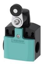
Position switch Plastic 50 mm, Increased corrosion protection Device connection 2 x (M20 x 1.5) 1 NO/1 NC snap-action contacts twist lever metal lever with plastic roller 19 mm functional at -40  $^{\circ}\text{C}$  Shock and vibration test according to EN 61373, Category 1B
