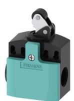
position switch plastic enclosure 50 mm, device connection 2 x (M20 x 1.5) 1 NO/1 NC slow-action contacts, roller lever with plastic roller 13 mm
