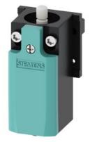
Position switch Plastic enclosure, 31 mm according to EN 50047 Control cabinet type 1 NO/1 NC snap-action contacts integrated (not replaceable) Rounded plunger Degree of protection IP40, with Self-sealing grommet Standard cover, turquoise With accessories: screws and mounting plate without locking sheet metal and seal
