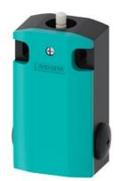
Basic switch for position switch 3SE5162 Metal enclosure XL, 56 mm wide Device connection  $3x(M20 \times 1.5)$  IP66/IP67 2 x (1 NO/2 NC) Slow-action contacts with make-before-break without actuator head with increased corrosion protection
