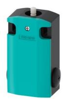
Position switch Basic switch Metal enclosure XL, 56 mm wide Increased corrosion protection Device connection 3 x (M20 x 1.5) 2 x (1 NO/1 NC) quick action contacts functional at -40  $^\circ$ C Shock and vibration test according to EN 61373, Category 1B
